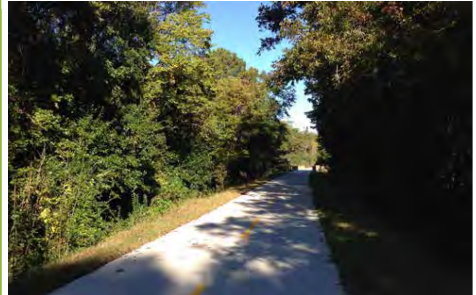
Multi-use trails with a 12-foot wide concrete surface provide for low long-term maintenance.
