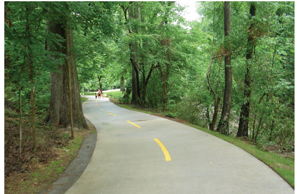
Sloping trail away from nearby creek into a gravel drain allows runoff to infiltrate under trail prior to entering creek.
